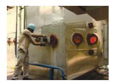
Extensive tests using this trial apparatus have been carried and once again, the results have been encouraging. Successful recirculation of the flue gas from the chimney has been achieved as has been the transition from air-coal combustion to oxy-coal combustion.  $NO_x$  and  $SO_2$  emission levels have been quantified for the purpose of comparisons and the optimum flue gas circulation for a favourable flame temperature determined.
