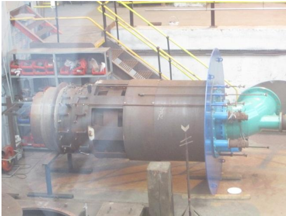
Single burner for 40 MW Oxyfuel Combustion
