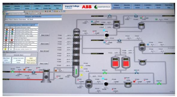
Figure 3: Schematic representation of stripper and reboiler.
