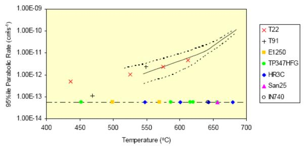
Figure 25: Corrosion studies with different material for oxy-coal combustion with El cerrejon coal.
