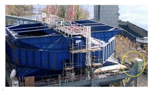
Figure 6: Rotating adsorption and desorption experimental set-up for post combustion CO<sub>2</sub> capture.
