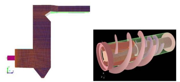
Figure 12: Combustion chamber geometry and burner configuration with meshing for CFD simulations.
