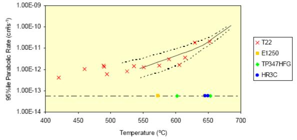
Figure 24: Corrosion studies with different material for air-coal combustion with El cerrejon coal.
