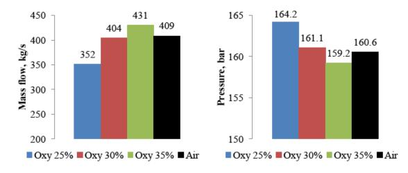
Figure 17: Predicted steam flows and pressures at superheater exit for air-coal and oxy-coal (at different O<sub>2</sub> concentration) combustion systems.
