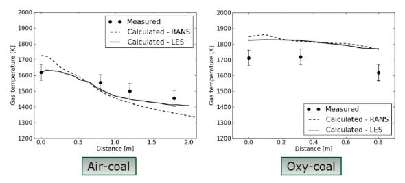
Figure 15: comparison of experimental and predicted gas temperature across the combustion chamber for air-coal and oxy-coal system
