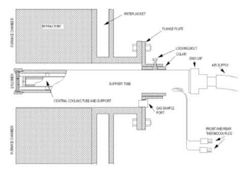
Figure 23: Corrosion test rod for testing different material in air-coal and oxy-coal combustion experimentation.
