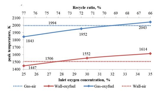
Figure 18: Predicted peak temperatures at wall and near combustion zone air-coal and oxy-coal (at different  $O_2$  concentration) combustion systems.
