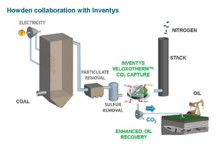
Figure 5: Schematic lay-out of post-combustion CO<sub>2</sub> capture from power plant.
