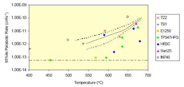
Figure 26: Corrosion studies with different material for oxy-coal combustion with Thoresby coal.
