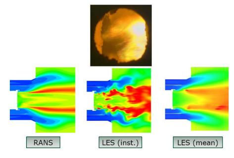
Figure 14: Comparison of predicted and experimental flame shape for oxy-fired coal combustion system.
