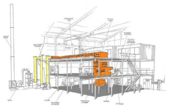
Figure 22: Schematic representation of E.ON's 1  $MW_{th}$  oxy-coal combustion test rig.
