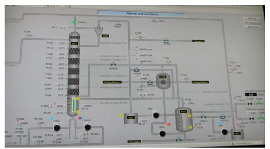
Figure 2: Schematic representation of absorber and gas recycle.
