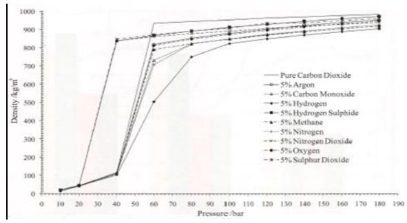
Figure 8: Effect of impurities on CO<sub>2</sub> compression pressure.
