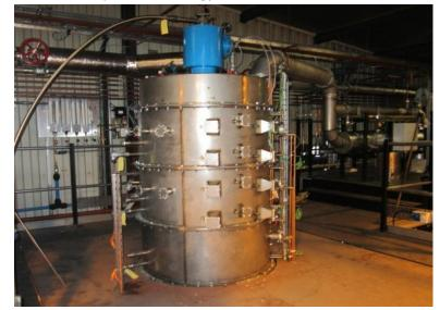
Figure 20: 250 kW vertically down fired oxy-fuel combustion chamber at PACT facilities, Sheffield.
