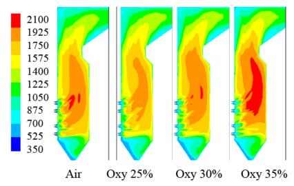
Figure 16: Comparison of temperature profiles for air-coal and oxy-coal systems.
